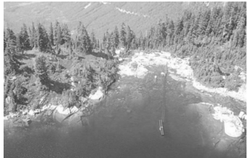
Figure 7-6 A 400 metre long salmon spawning channel constructed as part of the Sechelt Creek hydropower development in British Columbia, Canada. The scheme was developed in close collaboration with the local indigenous community. An aerial view of the headwater intake for the powerplant is shown (right).
