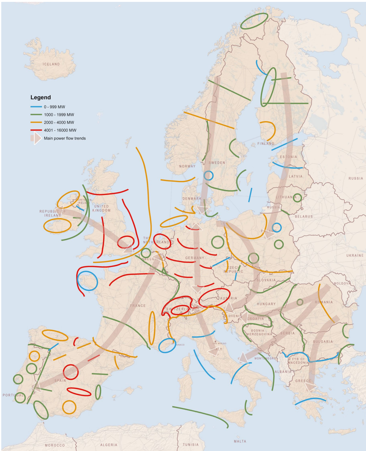
Figure 7.5: Grid Transfer Capability increases
