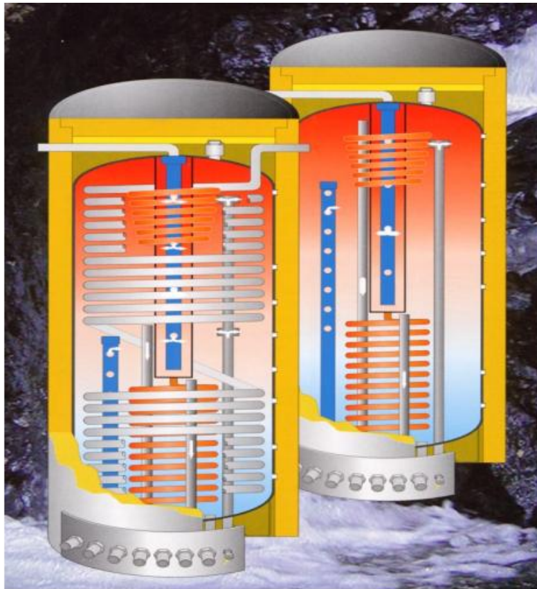
Fig. 5a: Water storage with thermal stratification
