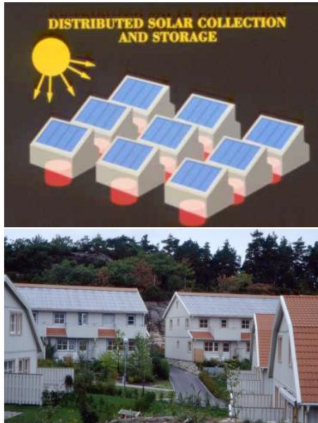
Fig. 21: Decentralised solar thermal storage
