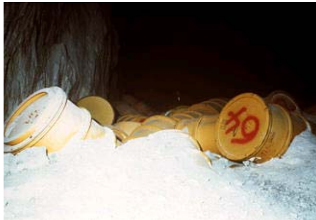
Figure 4 Damaged nuclear waste containers at the Asse facility. Containers were rusting due to brine inflow, threatening groundwater security
