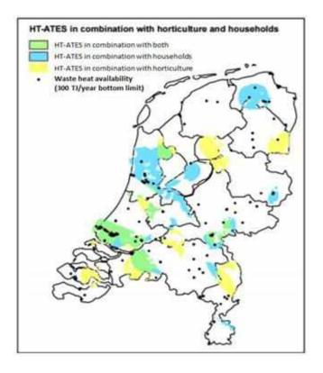
Figure 2: map indicating where suitable subsurface and surface conditions for HT-ATES overlap [14]
