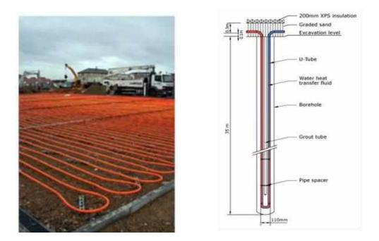
Figure 3-4: Left, horizontal U-tubes. Right, a cross-section of vertical borehole heat exchanger [4]
