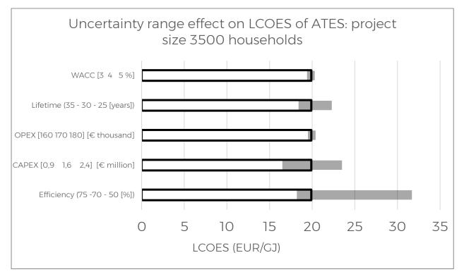
For ATES, the spread in efficiency is large. Systems can perform much worse than designed and therefore the efficiency can be much lower. This means costs can be much higher for ATES is efficiency is lower than expected. CAPEX is also a source of considerable variance. Since the CAPEX is relatively low, the WACC is only of small influence.
