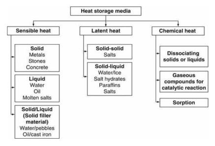
Figure 2-3: thermal energy storage classification [30]
