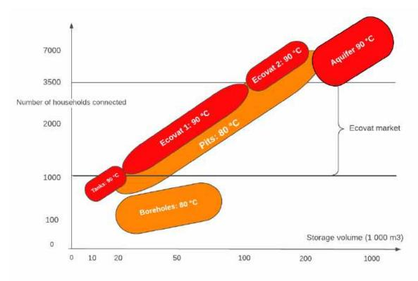
Figure 0-3: Suitable project sizes for high-temperature seasonal ATES, BTES, PTES, TTES and Ecovat.
