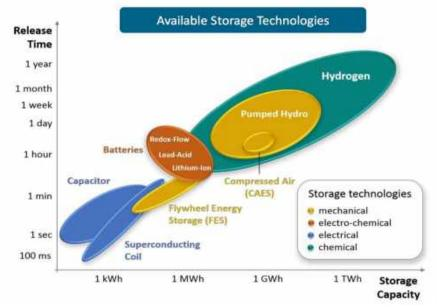
Figure 2-1: Electrical energy storage technologies and their range of applications
