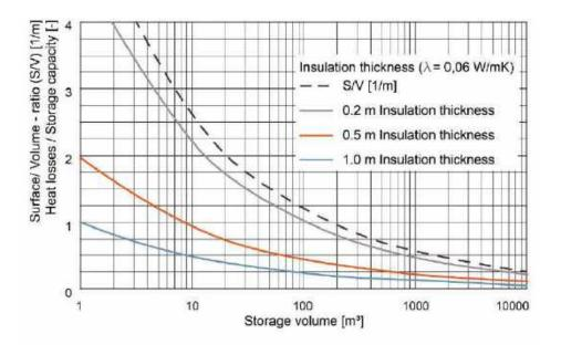
Figure 12: Ratio of heat losses to storage capacity ratio versus storage volume in m<sup>3</sup> for a storage duration of 6 months and a storage temperature of 40 K above ambient temperature [2]
