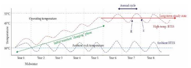
Figure 6: Temperature evolution of BTES for low and medium temperature BTES operation [21].
