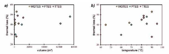
Figure 13: Performance of present storage systems in relation to volume (a) and operation temperature level (b). WGTES = Water-Gravel Thermal Energy Storage [28].
