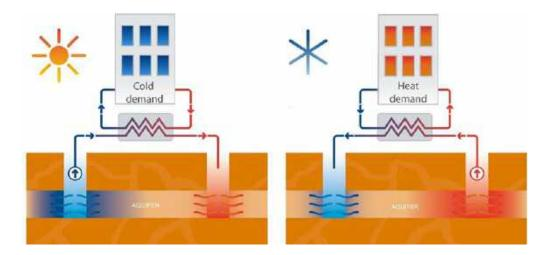
Figure 3-2 Workings of ATES two well system (IF technology) <u>https://www.iftechnology.nl/aquifer-thermal-energy-storage-</u> <u>wko-in-dutch-is-catching-on-in-japan</u>
