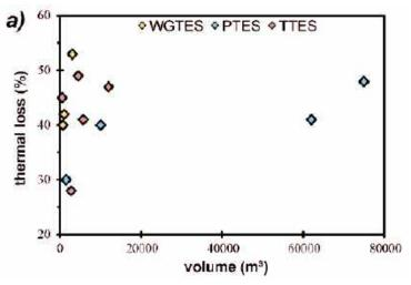
Figure 8: Thermal losses as function of storage volume for Pits, Tanks and Water-gravel storages
