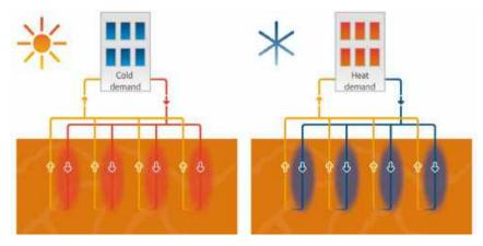
Figure 3-6 Working principle of seasonal BTES storage https://www.iftechnology.com/borehole-thermal-energy-storage/
