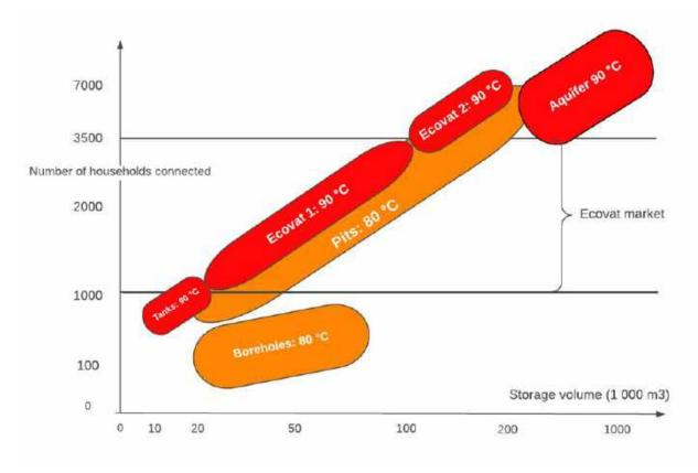
Figure 0-3: LSSTES technologies and their range of high-temperature storage application
