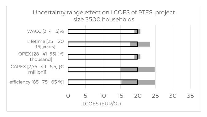
PTES has quite a large spread in lifetime (relatively), because the liner materials are currently not sufficiently resistance to high-temperature exposure. The low lifetime also causes the uncertainty in CAPEX to have a strong effect on the LCOES. PTES systems also show high variance in efficiency, which also causes high variability in the LCOES.
