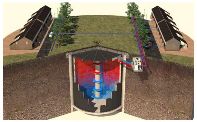
Figure Ecovat tank and connection to heating infrastructure schematic
