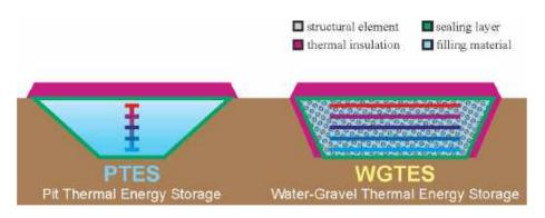
Figure 3-11: Subdivision of pit storage systems according to storage medium [28]
