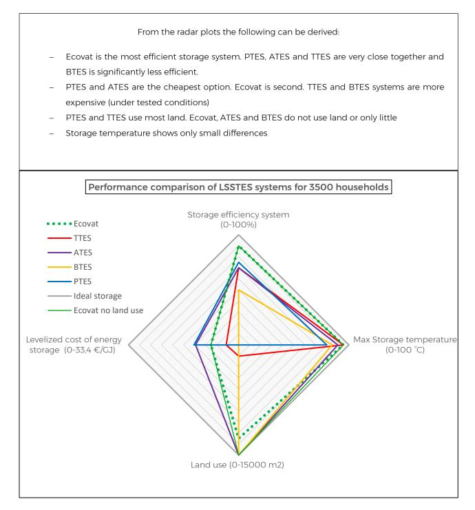
Figure 4-3: Enlarged radar plot of all LSSTES systems and the ideal storage unit
