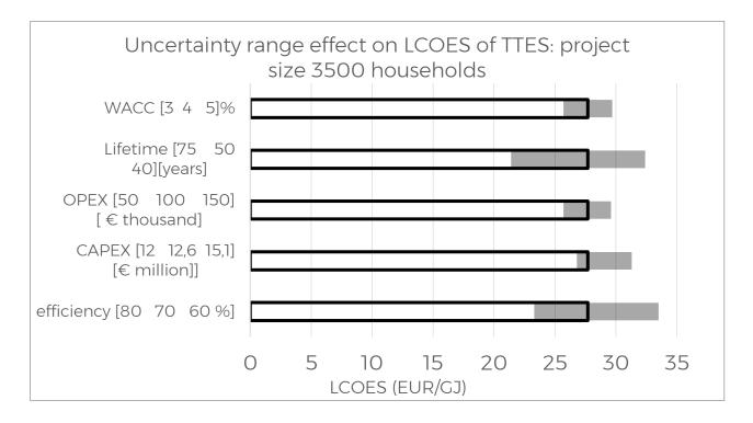
TTES is similar to Ecovat in terms of the high spread in costs due to lifetime uncertainty. TTES systems have a larger spread in the efficiency, which is also a source of large cost variability.
