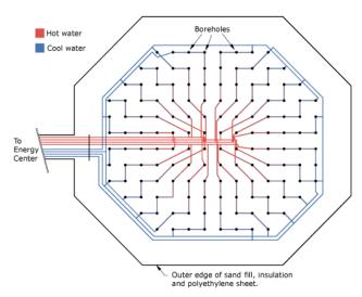
Figure 3-5: Top view of BTES heat exchanger pipes [4]
