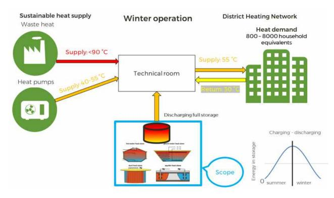
Figure 0-2: Winter operation and state of charge of the LSSTES within the DHN
