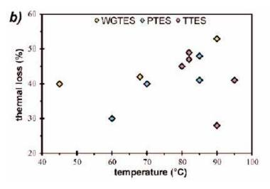
Figure 9: Thermal losses of Pits, Tanks, and Water-gravel storages as function of storage temperature
