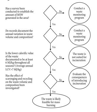
Assumptions regarding the delivery of combustible industrial and commercial waste to an incineration plant should be founded on an assessment of positive and negative incentives for the various stakeholders to dispose of their waste at the incineration facility.
