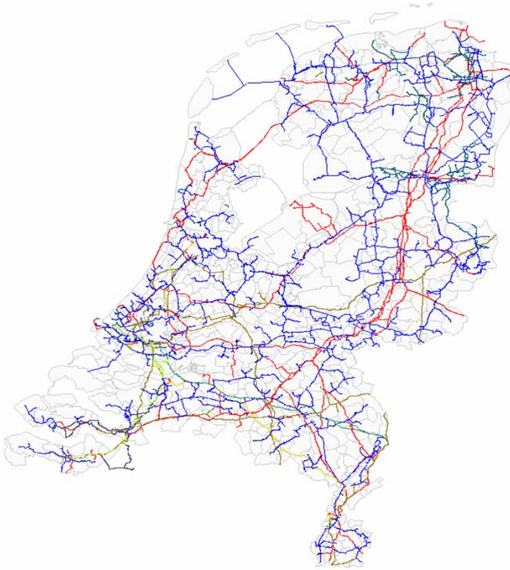
Figure 1 The existing pipeline corridors in the Netherlands (in red gas 60 bar, in blue gas 40 bar, in green oil and in yellow chemicals). Source: (Speel, 2007).
