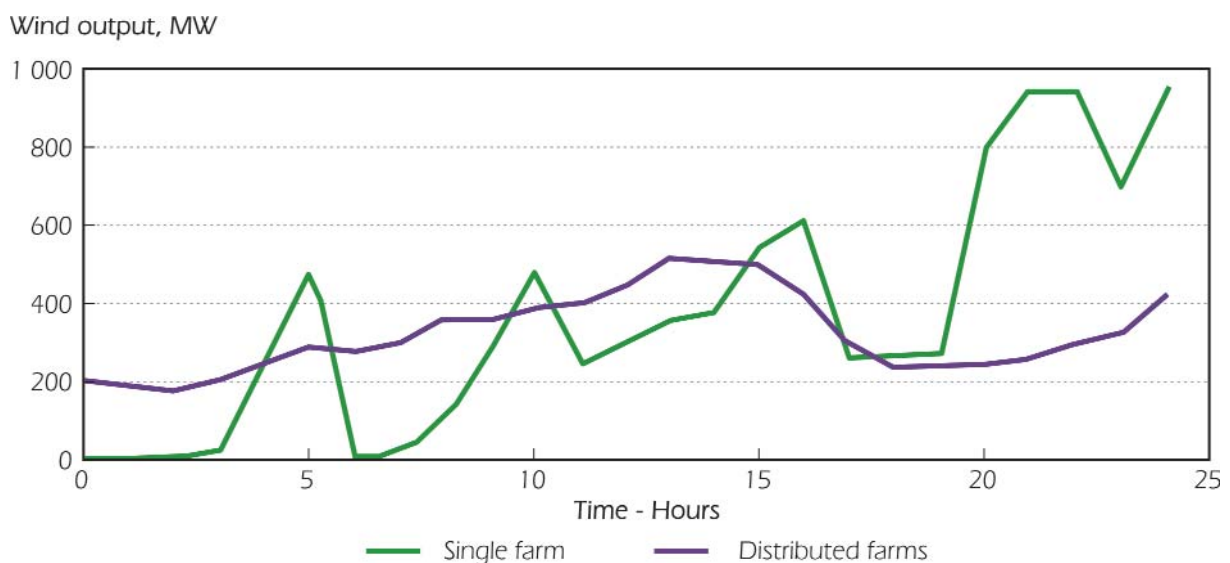
Figure 3: The smoothing effects of geographical dispersion of a single wind farm and distributed wind farms, both rated at 1000MW (Mott MacDonald 2003:8)
