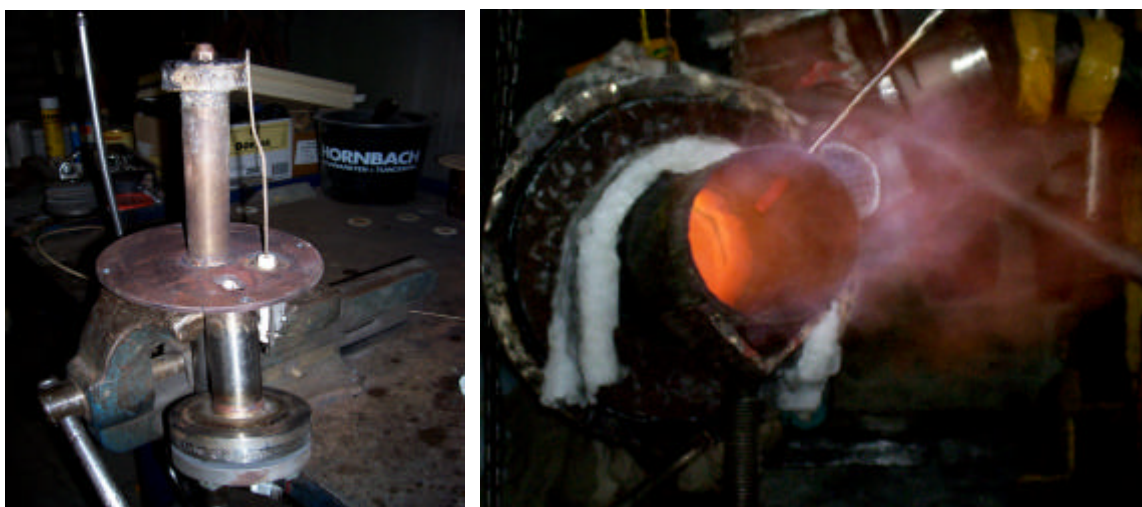
Figure 5-20 Left: picture of the dual-fuel natural gas and glycerin injector after operation Right: experiments of the RCG crude bio-fuel combustor running on crude glycerin
