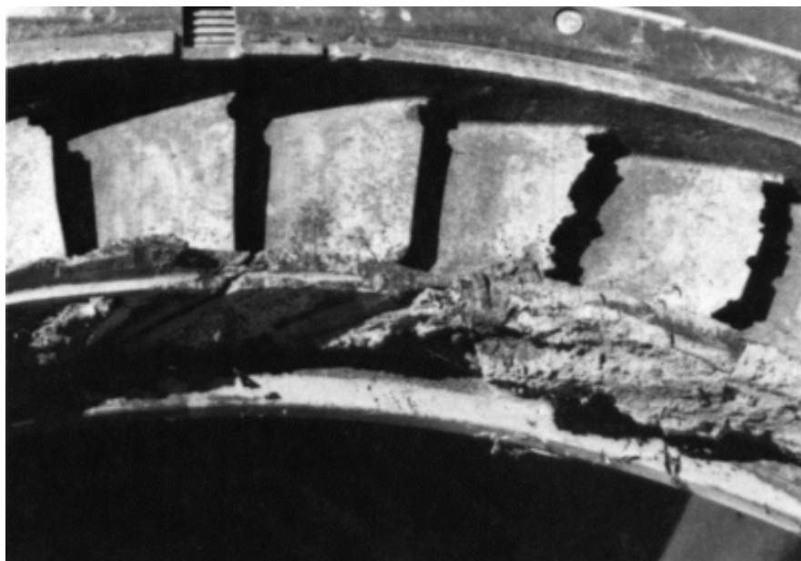
Figure 5-10 Damage of turbine guide vanes due to combustion problems ( www.gpal.co.uk )
